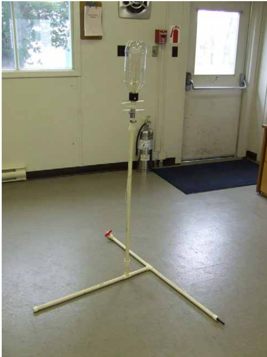
Figure 33-A Assembled Water Rocket Launch System
