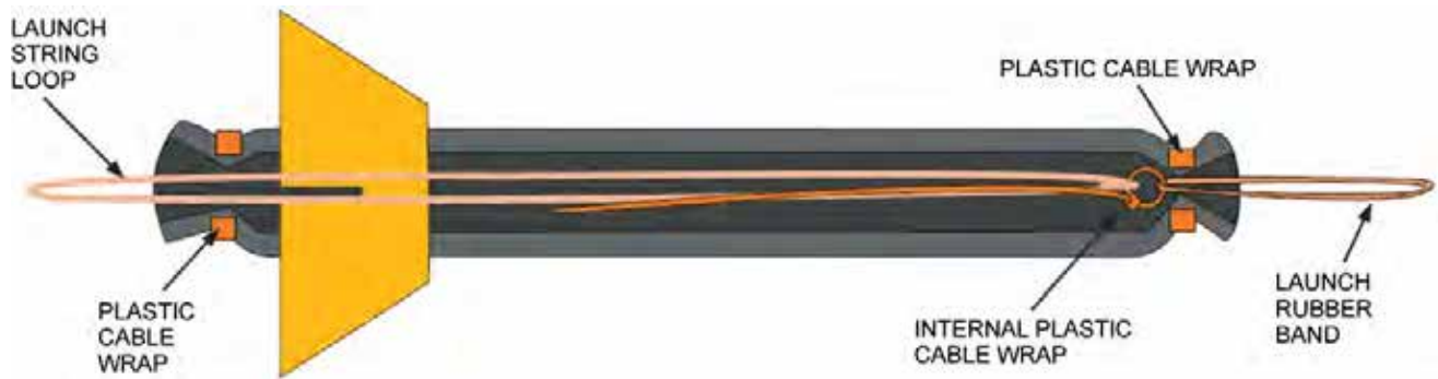
Figure 1 Exploded View of the Foam Rocket
