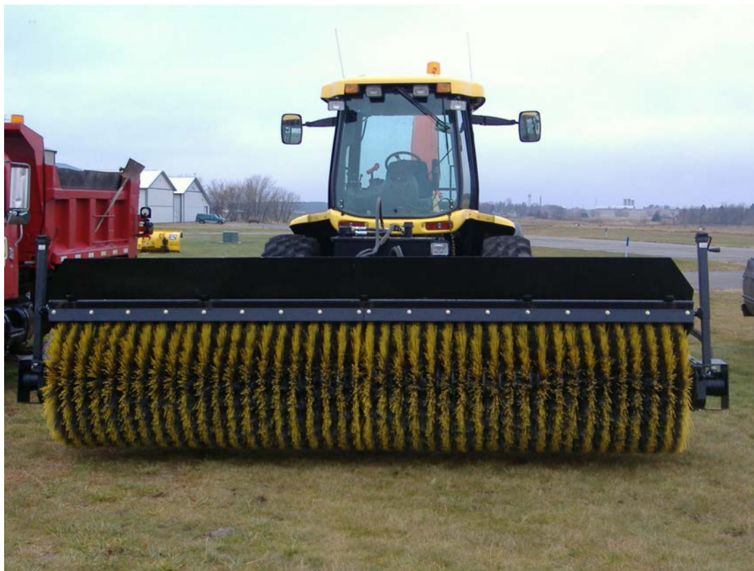
Figure 16E-7 Front Mounted Sweeper
