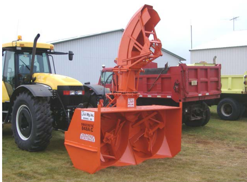
Figure 16E-10 Front Mounted Snow Blower (Mounted on a Tractor)
