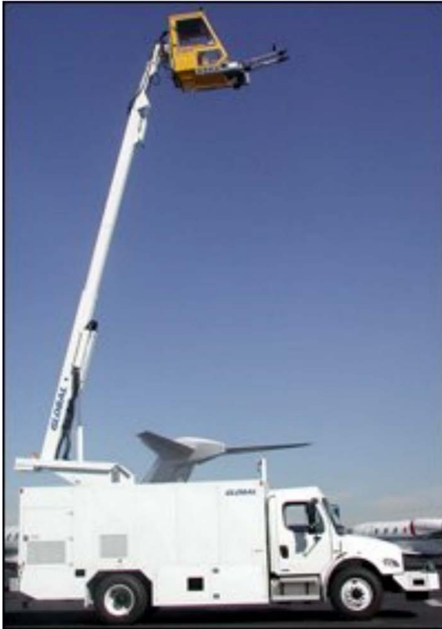
Figure 16E-5 A De-Icing Truck Used at an Aerodrome
