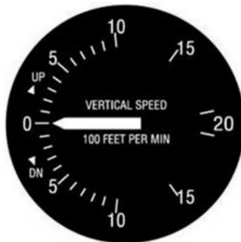
Figure 17B-3 Vertical Speed Indicator Parts
