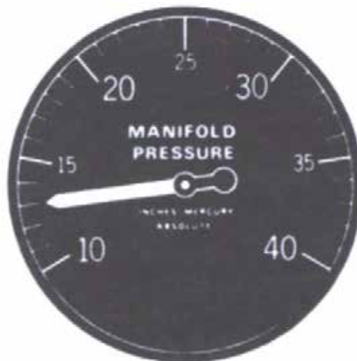
Figure A-4 Manifold Pressure Gauge
