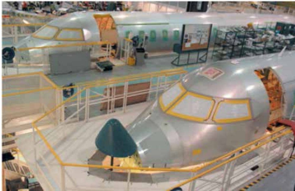
Figure A-9 Bombardier CRJ700 Fuselage Assembly
