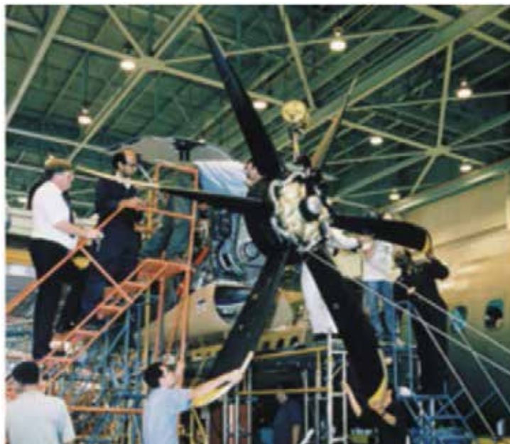
Figure A-8 Bombardier QR 400 Engine Assembly
