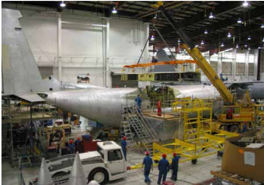
Figure A-1 Rebuilding a C-130 Centre Wing
