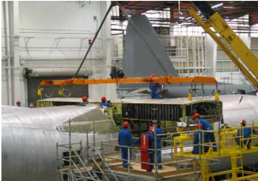
Figure A-3 Positioning a C-130 Centre Wing
