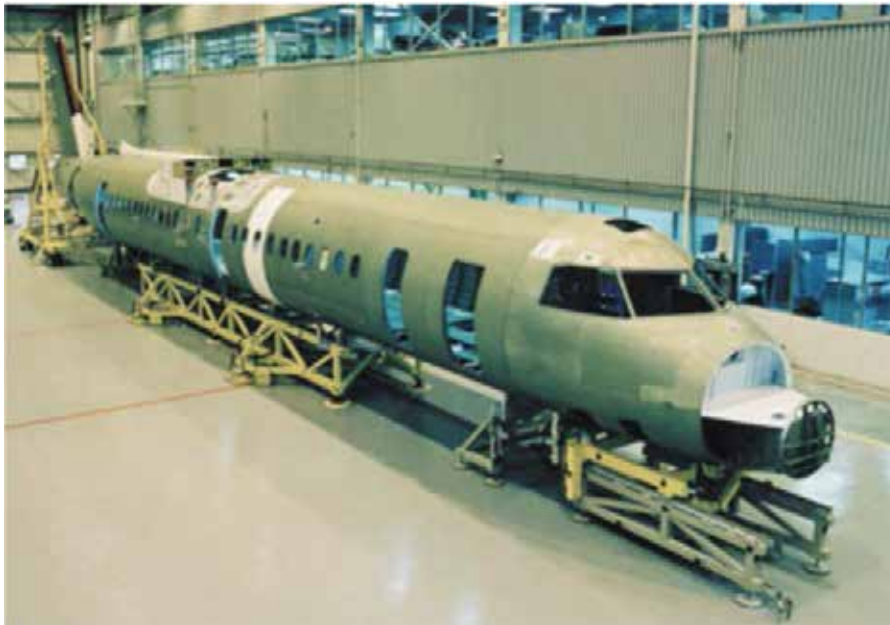
Figure A-4 Bombardier QR 400 Fuselage Assembly
