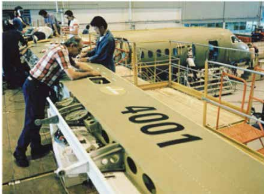
Figure A-5 Bombardier QR 400 Wing Assembly
